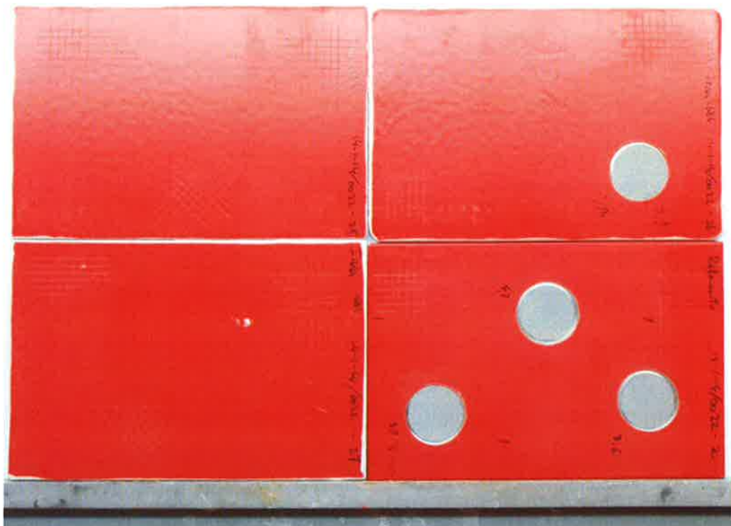
Photo 4: Panels after 168 hours H 2 SO 4 Immersion Test
