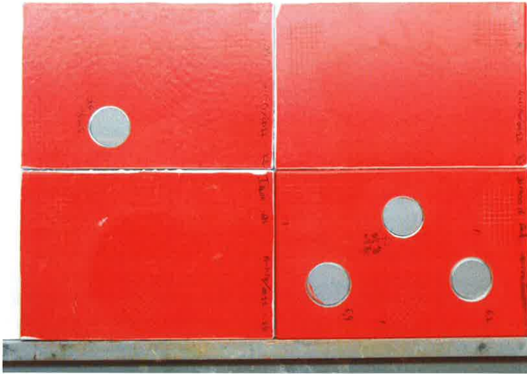
Photo 3: Panels after 168 hours NaOH Immersion Test
