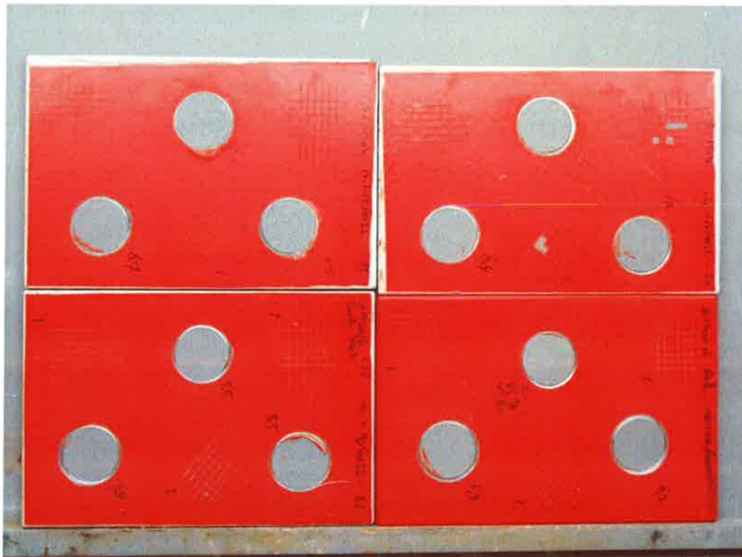
Photo 2: Panels after 720 hours Condensation Test.
