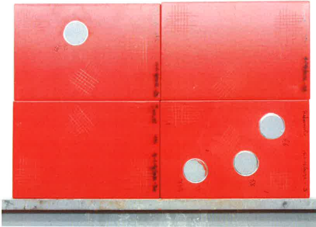
Photo 5: Panels after 168 hours Mineral Spirit Immersion Test.
