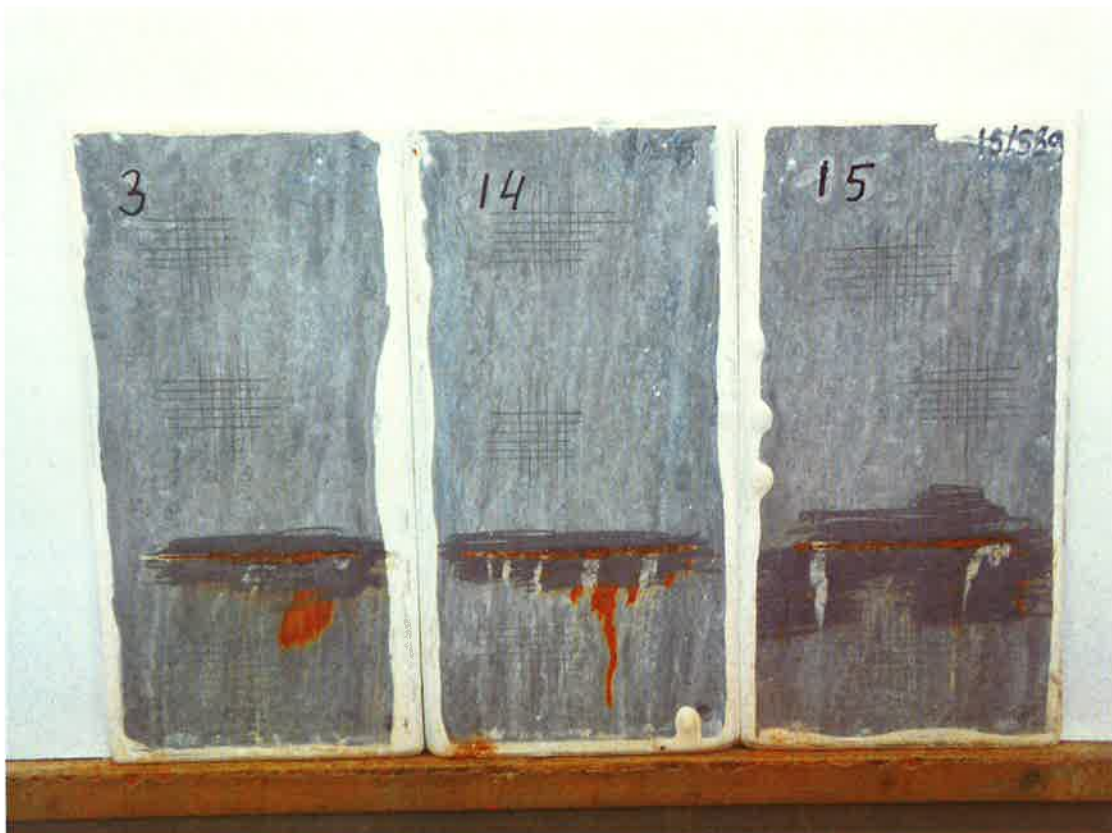
Photo 2: Panels 3, 14 and 15 after 1440 hours Neutral Salt Spray test.
