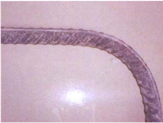
GALVATOR ® after 48 hr. salt spray
