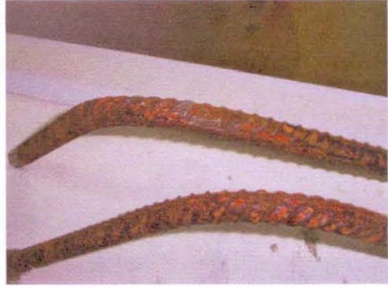
Carbon steel Rebars after 48 hr. salt pray
