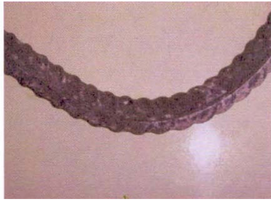
GALVATOR ® after 48 hr. salt spray
